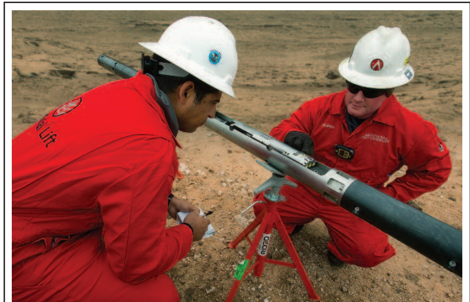
Artificial Lift Company's Advantage™ rigless ESP system is especially appropriate for wells located offshore or at remote, difficult to reach sites. The company explains that the equipment can be deployed with a crane and a slickline unit rather than a workover rig, minimizing infrastructure needs and the operational footprint.
